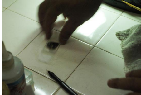
Gambar 1.12 Proses penempelan cover glass
